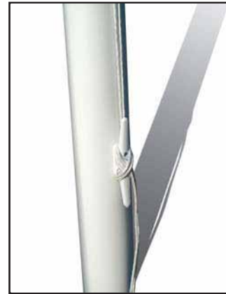
Bitt with an external rope
